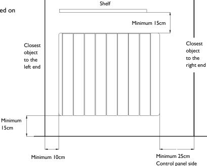
Position and fix the brackets at the correct distance from the floor. It is possible to use the radiator as measuring unit by positioning it on two polyester package elements and placing two supports above as indicated on the figure:
