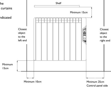
Position and fix the brackets at the correct distance from the floor. It is possible to use the radiator as measuring unit by positioning it on two polyester package elements and placing two supports above as indicated on the figure:
