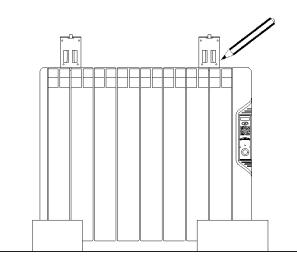
Mark the fixing points on the wall using a pencil through the two fixing holes in the square brackets and perform corresponding bores.
