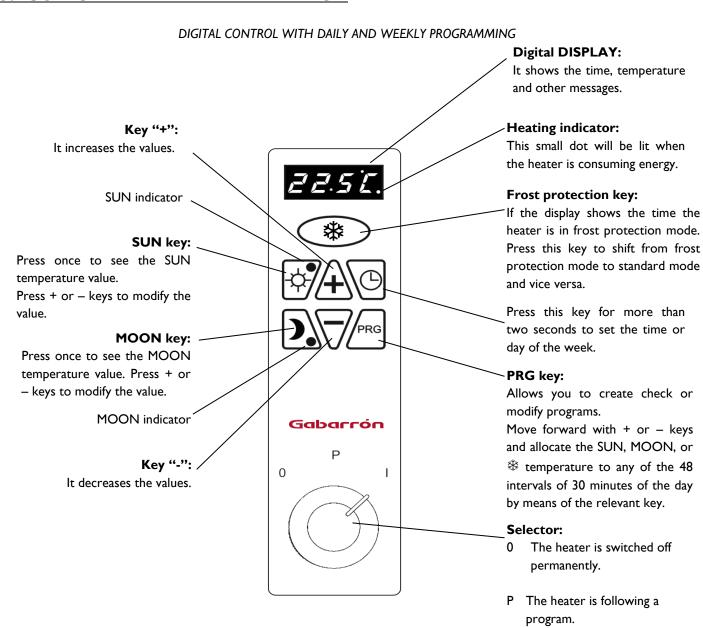
RFE Plus models have built in an electronic thermostat with a sensibility of 0.1  $^{\circ}$ C. It is possible to set temperatures with an accuracy of 0.5  $^{\circ}$ C.
