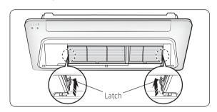
2 Open the screw cover on the air outlet, insert and fasten the panel fixing screws. If the screws are not fastened completely, it may produce a gap between the indoor unit and the panel, resulting in condensation.
